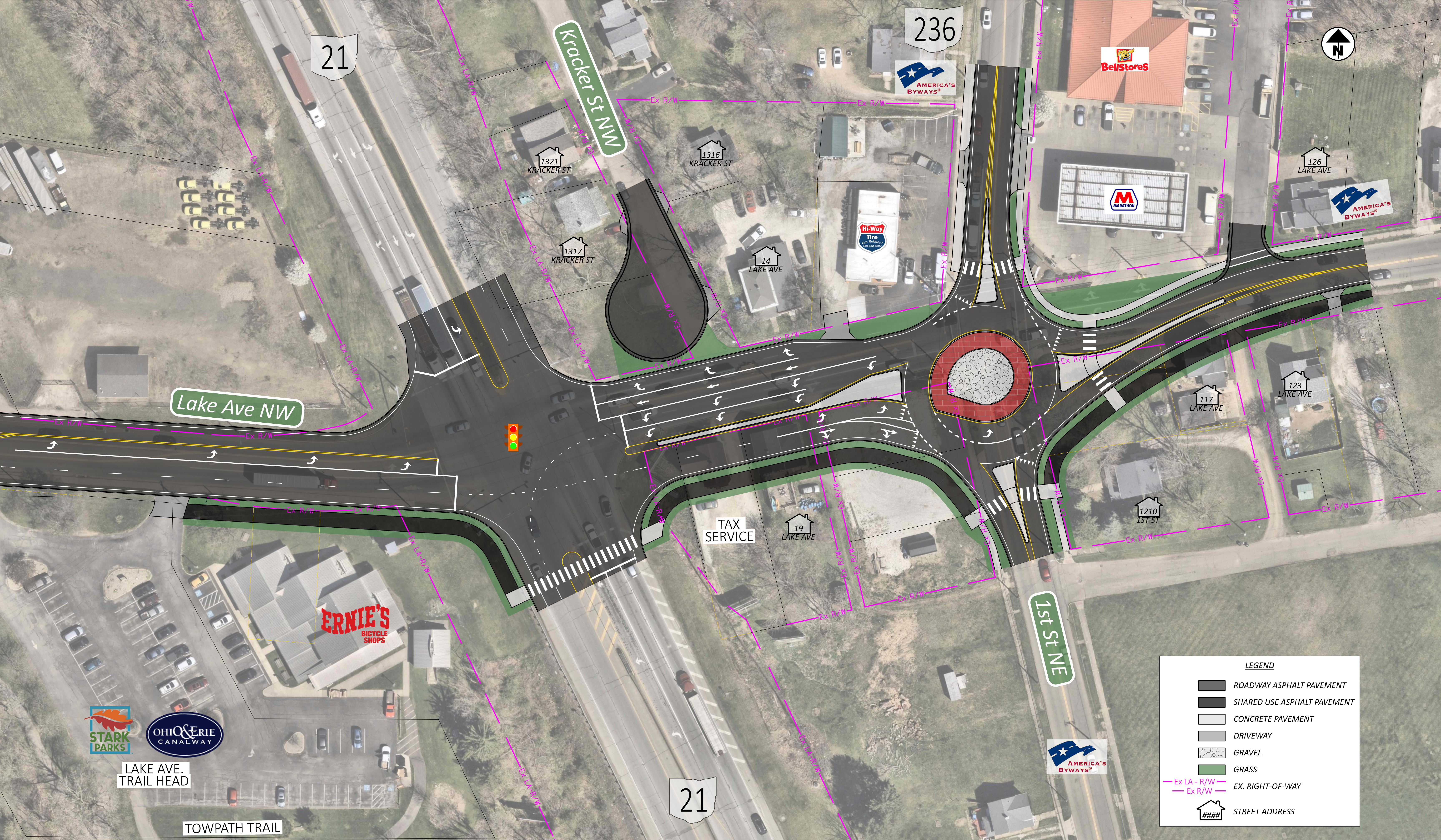
STA-21-10.46 SR-21 & LAKE AVENUE IMPROVEMENTS (PID 122272) ALTERNATIVE 5 (VIEW 2) TRAFFIC SIGNAL UPGRADES, ROUNDABOUT, AND ADDITIONAL TURN LANES WITH SHARED USE PATH
