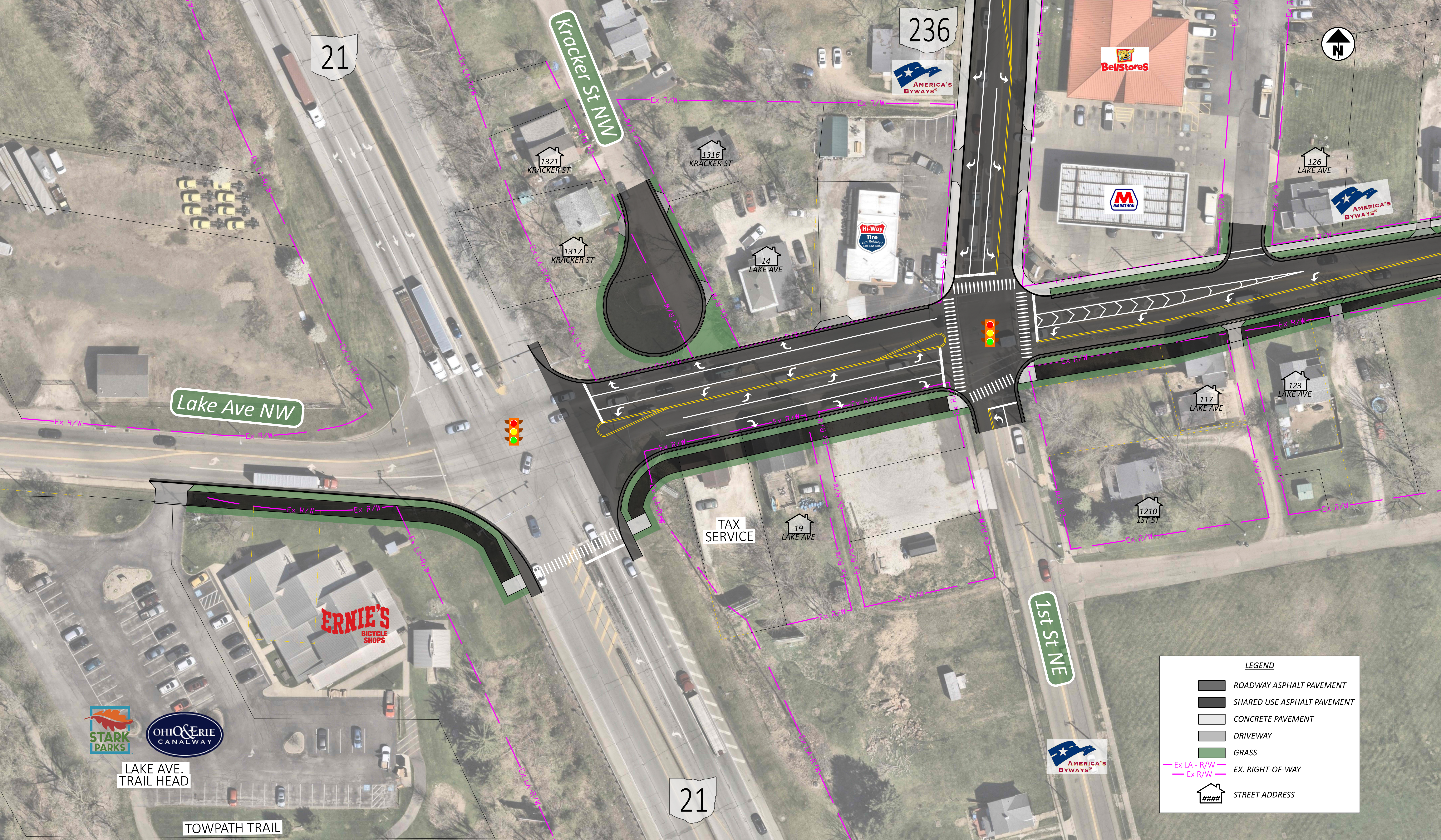
STA-21-10.46 SR-21 & LAKE AVENUE IMPROVEMENTS (PID 122272) ALTERNATIVE 4 (VIEW 2) TRAFFIC SIGNAL UPGRADES AND ADDITIONAL TURN LANES WITH SHARED USE PATH
