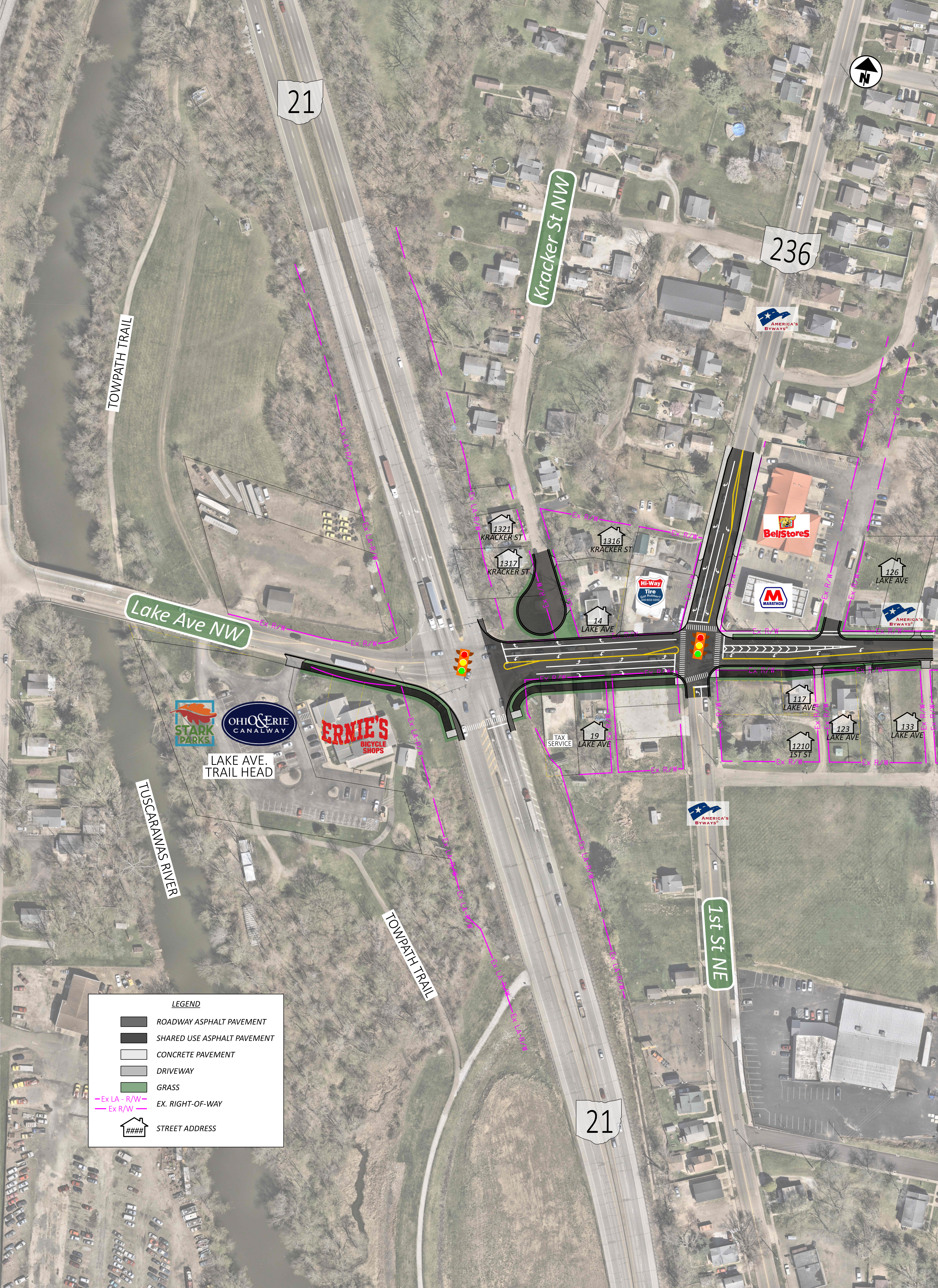
STA-21-10.46 SR-21 & LAKE AVENUE IMPROVEMENTS (PID 122272) ALTERNATIVE 4 (VIEW 1) TRAFFIC SIGNAL UPGRADES AND ADDITIONAL TURN LANES WITH SHARED USE PATH
